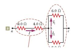
Use  $(R = \Delta V/I)$  and the result from part (A) to find the current in the 8.0- $\Omega$  and 4.0- $\Omega$  resistors:
